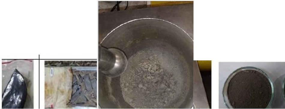
Figure 18. Rock samples of La Luna Formation used to prepare a synthetic flowback on a laboratory scale.
